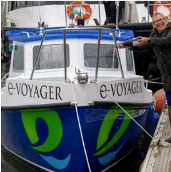
E-Voyager is a refit of an old diesel ferry and uses 2nd life batteries
