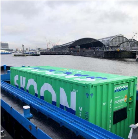
Skoon floating battery terminal to charge electric boats in Amsterdam canals
