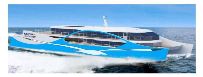
In February 2020, South Korea commissioned Haemin Heavy Industries, a small aluminium-vessel shipyard in Busan to build a 100 PAX, all-electric ferry for the Busan Port Authority. The 40-m catamaran will commute between Busan's North and South ports, a one-hour round voyage at an average operating speed of 13 knots, multiple times a day. ABB will provide the DC grid distribution system and the power and energy management system for the propulsion and all auxiliary power loads.
