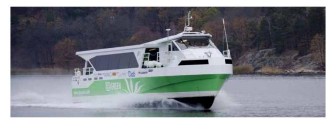
In 2014, the Swedish companies Echandia and Green City Ferries launched the retrofitted all-electric passenger ferry Movitz. With a 200-kWh battery and a diesel engine for back-up, Movitz could operate as a commuter in Stockholm for 1 ½ hours and recharge in 15 minutes.
